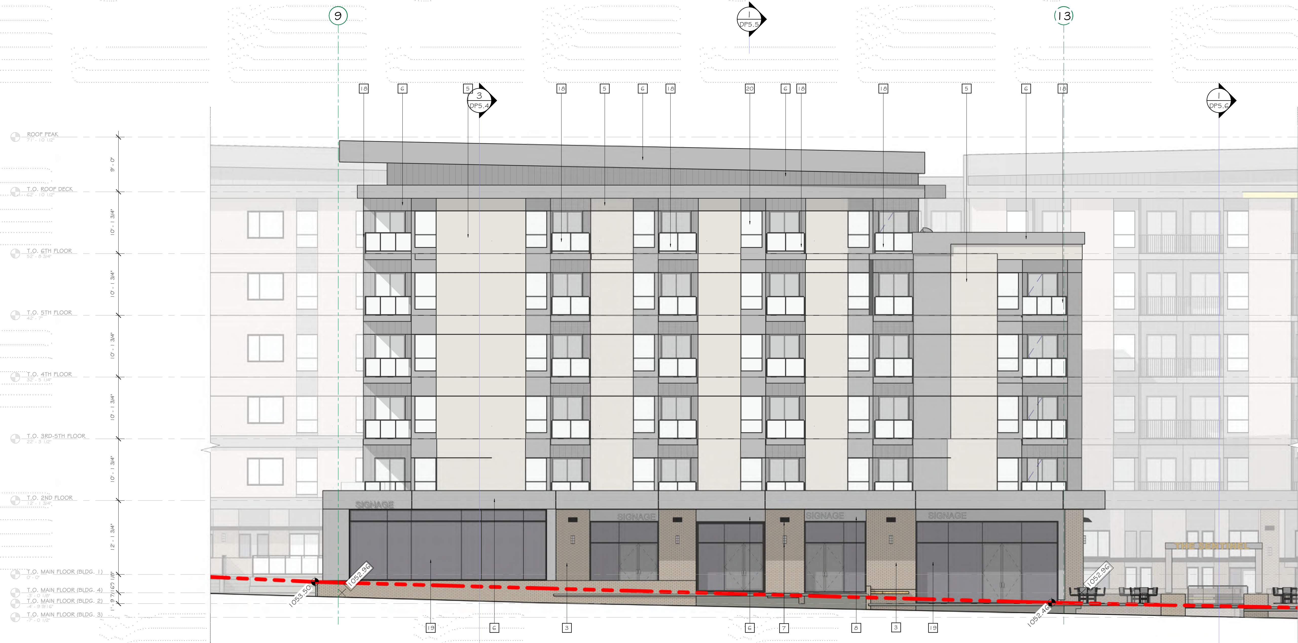
SOUTH ELEVATION BUILDING 2 1/8" = 1'-0"
